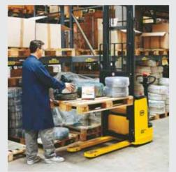
**Traction group**: The brad-new traction motor introduces the innovative 1 kW power AC 3-phase technology. The electronic traction control allows energy recovery when releasing the butterfly, minimizing energy consumption requested to the battery, motor and brake heating and the necessary stopping distance. The pivoting wheel is easily adjustable in order to maintain perfect contact with the floor and maximum stability
